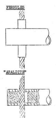
Used for solid or hollow rungs. Two ferrules of annealed aluminium alloy are placed one either side of the rung and compressed by means of a die. The soft metal being forced into the interstices of the wire rope, thus securing the rung.
