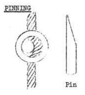
This method utilises a rung having an internal diameter a little larger than the pin used. The fastening is effected by trapping the wire rope between the pin and the internal wall of the rung by driving a chamfered pin up the bore of the tube.
